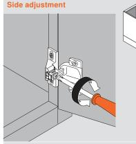
Side adjustment is possible on all COMPACT hinges. COMPACT 38N, 39C and 38C have cam side adjustment.
