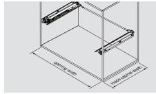
**NOTE:** Recommended for opening widths **610** (24") to **1369** (53-29/32") wide
