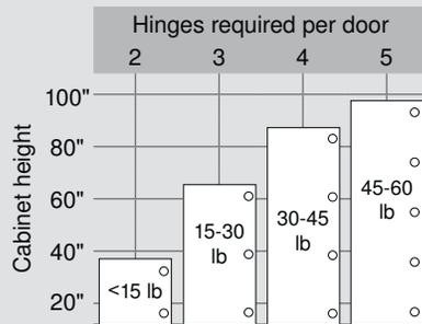
This chart can serve as a guide for determining the number of hinges per door. Note that door weight can also determine the number of hinges required.
