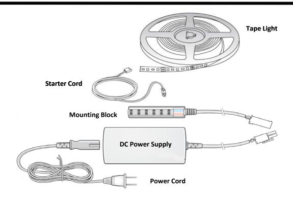
To design your FlexTape lighting system, start with the fixture. The FlexTape light is sold in a 20 ft roll.To choose your required DC Power Supply, add up the wattage of the desired length of Flextape.
