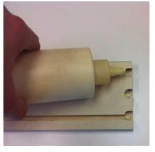
Apply Glue to the current Dovetail pocket ready to be connected.
