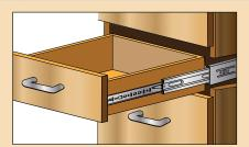
When inserting the drawer, first be sure the ball bearing retainers in the cabinet member are fully forward. Insert the drawer member into the cabinet member. Push the drawer in until it is completely closed; the Easy-Close mechanism will click and engage.
