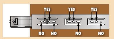
ALWAYS USE THE SYSTEM HOLES OR MOUNTING HOLES AT THE ENDS
