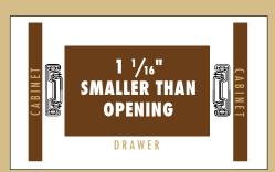
THE SLIDES WILL NOT FUNCTION PROPERLY IF THE SIDE SPACE IS LESS THAN .50".
